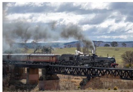
Heritage Garratt 6029 showing how the weight and driving forces are spread over numerous wheels in its 30-metre length. Its inaugural workings in 1953 were on Enfield-Broadmeadow runs. Source: David Patterson.
