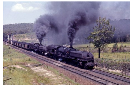
Double-heading Garratts hauling a heavy coal train out of Fassifern Station. Source: Steam Train Pics.
