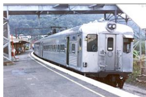
A 'U boat' interurban train built by Commonwealth Engineering in N.S.W., using Metropolitan-Vickers electrical equipment from Britain, arriving at Hawkesbury River Station. Some had operational lives of up to 38 years before retirement in 1996. Source: Stephen Halgren.
