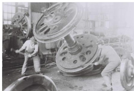
Workers in the 1950s removing a tyre from a C38 wheelset at Cardiff Railway Workshops established in 1928. Steam, diesel and electric locomotives have been maintained at the facility moved from public to private hands. Source Lake Macquarie Library.
