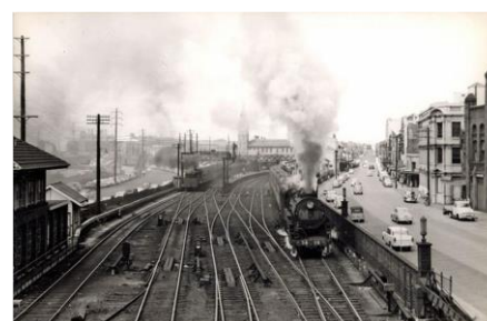
A pre-electrification Newcastle Rail Yard dominated by steam as a tank engine waits to haul out a Hunter Region train with wooden carriages while 3830 with 'The Flyer' builds up speed with an air-conditioned steel consist of cars trailing. Source: Pinterest .
