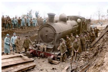
The end of the line – a colourised original photo of the challenges faced by all sides operating railways on the Western Front in the Great War. British and French troops try to dig a Belgian Type 30 locomotive out of the mud. Source: Bing Images.
