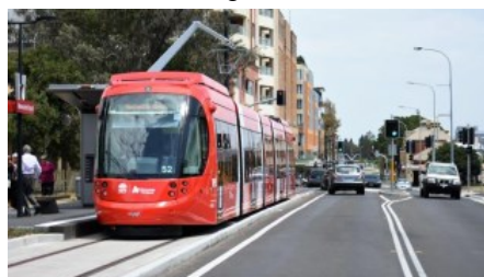
The light rail car with pantograph up connecting to the power to recharge batteries at Newcastle Beach stop. Source: Ron Johnson.
