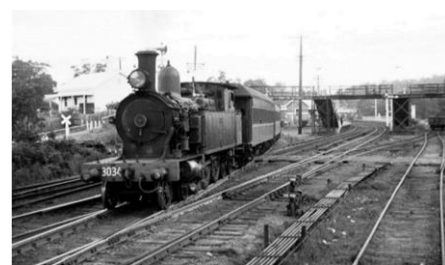
A 30-class tank engine with a trail of wooden 'Yankee' End Platform Carriages crosses from the Toronto Branch Line onto Main Northern Line at Fassifern Station in 1967. Source: Chris Nelson.
