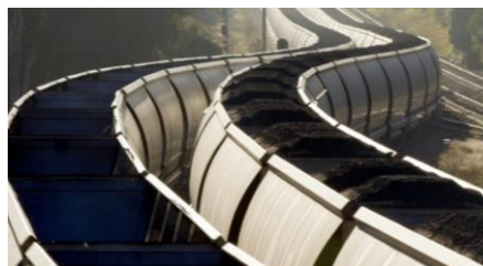
Railway rivers of coal flow down the Hunter Valley railway network and out of the Port of Newcastle. A rake of empty wagons heading back to the collieries snakes past a heavily-loaded rake heading to port. Source: Australian Financial Review .
