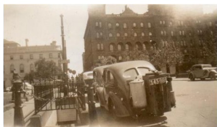
Motive vehicle with a charcoal burner fitted during WW2. Source: Monica Lynch.
