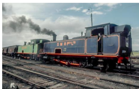
SMR tank locomotives double heading a coal train in reverse. Source: Brett Kavangh.
