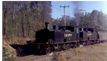
SMR 10-class tank locomotives working hard double-heading a heavy coal train. Source: Australian Steam .
