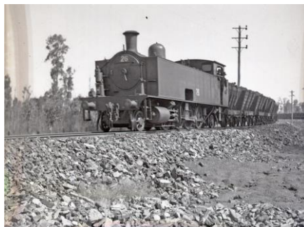
An SMR 10-class tank locomotive with a wooden hopper coal train. Source: Flickr .
