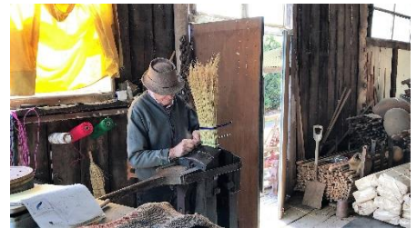
John at the compression bench to tightly gather the bunches for stitching firmly in place.
