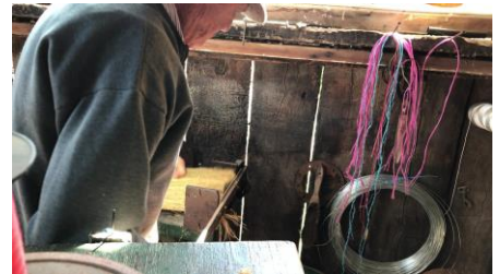
Transferred the broom to the guillotine for final shaping and trimming of the broom tip
