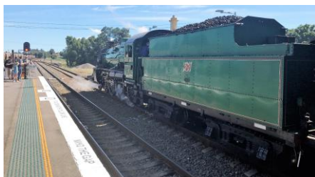
Locomotive 3642 is a two-cylinder, simple, non-condensing, coal-fired superheated, 4-6-0 36 class express passenger steam locomotive built for the New South Wales Government Railways in 1926 by Clyde Engineering.
