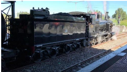
NSW Re-built 4-6-0 Steam Locomotive 3016 was originally built as 4-6-4 Tank Locomotive C30 in 1903. Today's appearance is much like the Rx steam locomotives of the same era in South Australia.
