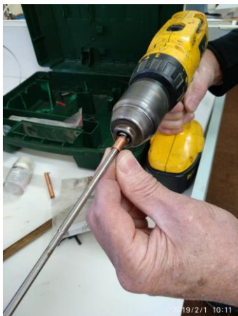
Coiling with the aid of a drill using a graduated mandrel made by Campbell.
