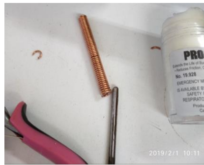
Coiled wire before cutting.
