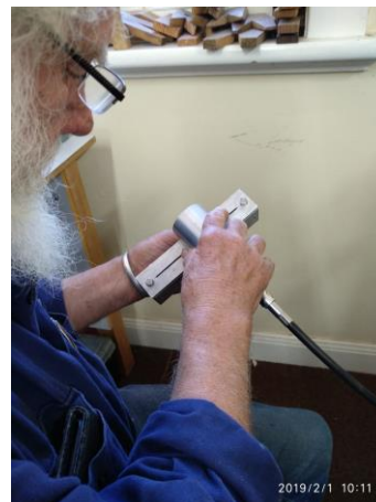
Campbell using his home-made guide and electric saw to cut jump rings.
