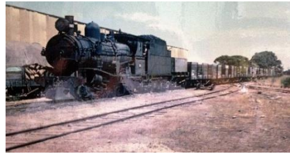
T 180 4-8-0 narrow gauge steam locomotive.
