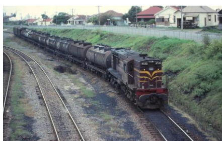
In 1981, the NSW Railways was still running relatively short trains such as this fuel consist entering Port Waratah pulled by a 45-class locomotive. Source: David Patterson.
