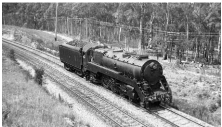
The fast 38-class locomotive 3815 running light between Fassifern and Awaba on the Main Northern Line in 1966. Source: David Patterson.
