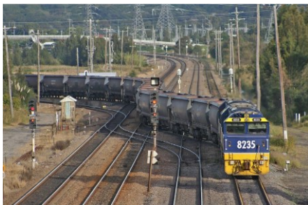
Before the flyover, a coal train crossing blocks multiple tracks. Source: Railpage.
