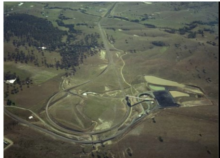
A rail balloon load-out loop at Mount Thorley Mine. Source: Brian Andrews.
