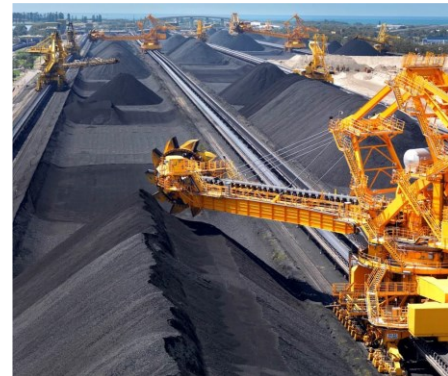
Stockpiling and reclaiming at Port Waratah Coal Terminal. Source: Angelfire.
