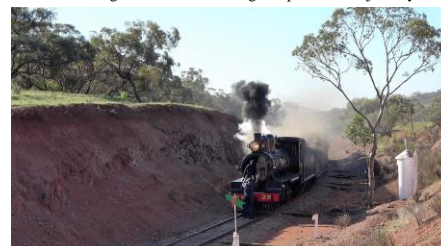
19. A slight blockage being dislodged in the smokebox.
