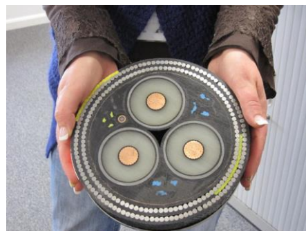
A cross-section of an undersea cable.
