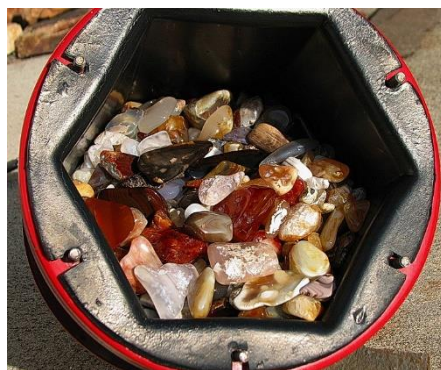
'Tumbled Agate and Jasper' tumble-polished gems inside a 15-pound rock tumbler barrel, by 88pathoofroad is licensed under CC BY-SA 3.0.
