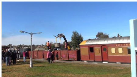
Coal and coal handling facilities are no longer available along the way so it is transported on the train and handled by local hired equipment.
