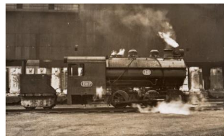
Narrow-gauge Loco No.30 made by BHP Newcastle for its own Steelworks. Source: NIHA.
