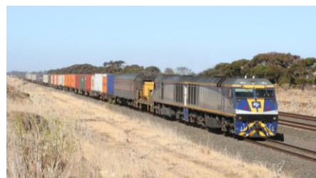
Another EL Locomotive geared to reach 140kph. Goninan built 14. Source: Wikipedia.
