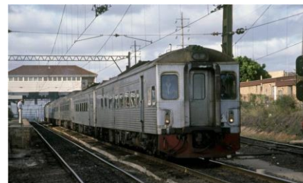
The ‘South Coast Daylight Express’ racing through Sutherland riding on Bradken cast bogies under its Tullouch and Budd rail cars. Source: David Patterson .
