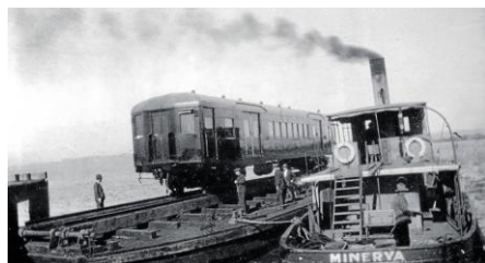
A completed Sydney electric railway carriage on a barge being transferred from assembly at Walsh Island State Dockyard. Source: Flickr.
