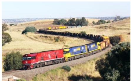
NR locomotives hauling a long freight train. Goninan built 120 NRs for National Rail. Source: Auscision Models.
