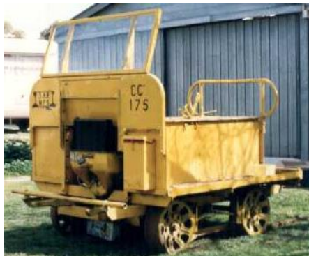
A Fairmont ST-2 section car used by SAR on the Eyre Peninsula.
