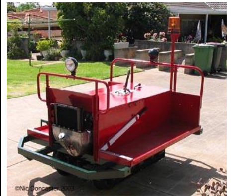
A former Queensland Railways Fairmont ST-2 section car converted from 42" to 24" line gauge and is owned by the Cobdogla Steam Friends, Cobdogla, South Australia.
