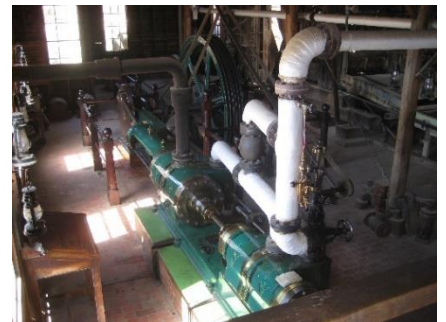
Steam engine in stamping battery.
