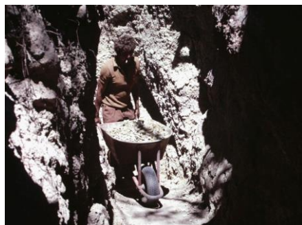
Dig a long shaft - and you end up with a long journey to the mullock heap. Discharge was made easy because Colin was working on ground that sloped down and away from his entrance.
