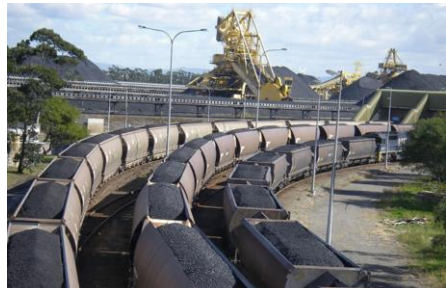
Coal feeding by rail to a loader in the modern Hunter Valley supply chain. Source: Australian Mining .
