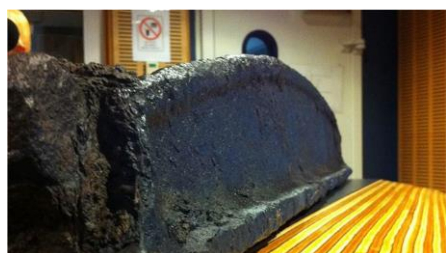
A remnant of the AA Company's first Fish Belly Railway line displayed in the Newcastle Museum, itself a former railway remnant – the Honeysuckle Workshops. The curve of the rail is likened to a fish belly and the rail is displayed upside down here. This rail installed in 1831, is like that used on the famous English Stockton to Darlington railway line of 1825. It is made of cast iron and hence quite brittle. Source: ABC .
