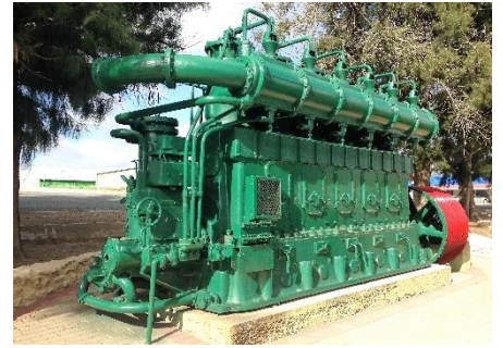
This, six cylinder, Worthington-Simpson, two-stroke, upright, marine type, crude oil pressure diesel engine was installed into the Waikerie Pumping Station along with three smaller units in 1928.
