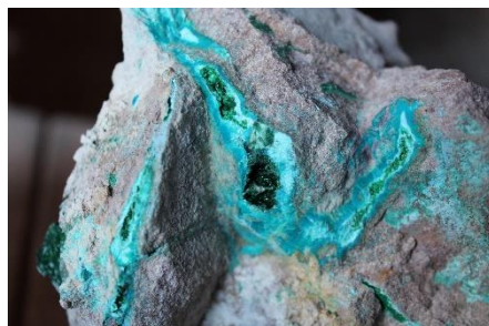
PHOTO 7. Atacamite in vughs overlaying malachite surrounded by chrysocolla. Atacamite crystals are also embedded in chrysocolla. Adit Drive, C4.
