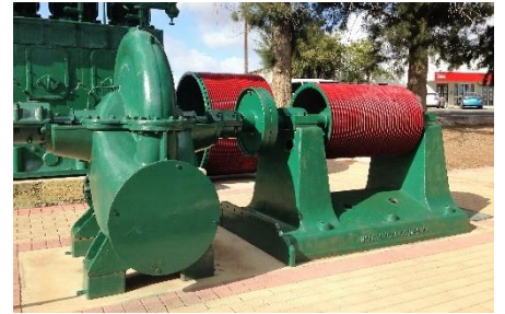
Pump driven via rope belts by the engine shown behind/above.
