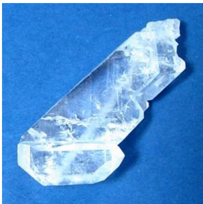
Faden Quartz - group of quartz crystals with a white thread-like zone running through the interior, with the crystals having formed around the thread axis.
