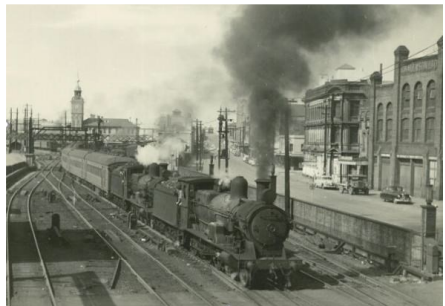
C32 class locomotives double-heading out of Newcastle in the 1950s. Source: A.R. Lyell .
