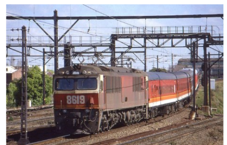
The Newcastle Flyer pulled by an 86-class electric locomotive. Source: Silverwater Plumbing.
