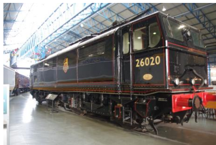
Electric locomotive, British Railways, Class 76 (EM1) Bo-Bo (Overhead) No. 26020, built at Gorton Works in 1951.
