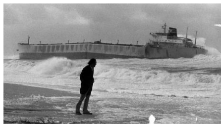
The 53,000 tonne Norwegian bulk carrier 'MV Sygna' with its spine shattered breaking up on Stockton Beach. Source: Pinterest.
