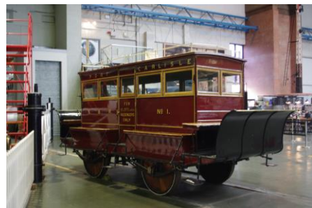
Dandy car, North British Railway, Port Carlisle Dandy Car (dark red horse drawn rail coach).
