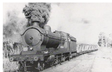
A J&A Brown Richmond Vale 2-8-0 ex-ROD British locomotives hauling a line of wooden coal wagons. Source: Wikipedia.
