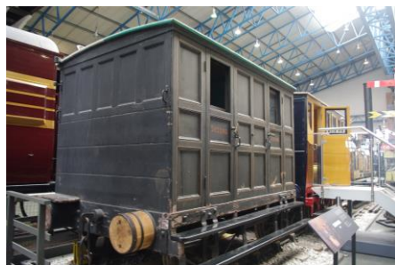
Railway carriage, four wheeled, 2nd class, Bodmin & Wadebridge Railway, built in 1834. Length over buffers: 17 ft.
