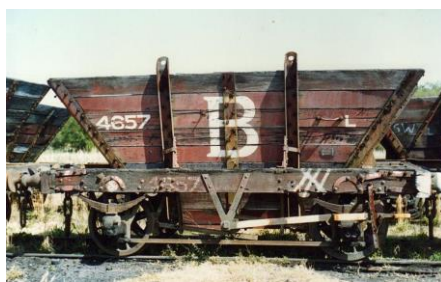
The primitive J&A Brown 10 tonne non-air braked railway coal hopper. Source: The Shed Rat.
