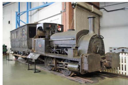
"Conserved but not restored" sums up this funny little Hebburn Works 0-4-0 industrial saddle tank steam engine built in 1874 by Black Hawthorn & Co. Ltd. of Gateshead.
