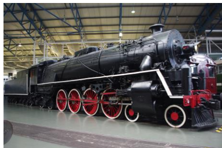
Steam locomotive KF class number 7, 4-8-4, Chinese Government Railways, designed by Colonel Kenneth Cantlie, built by Vulcan Foundry in 1935 (as number 607).
