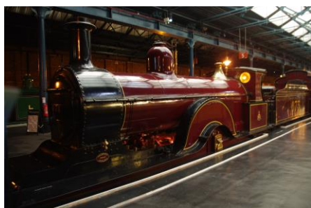
Steam locomotive, Midland Railway, 4-2-2 No 673, Midland Spinner, designed by S.W. Johnson, built at Derby in March 1897.
