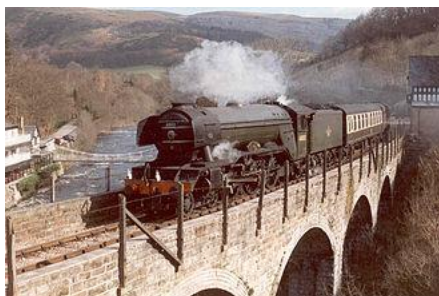
Flying Scotsman wearing its British Railways livery and numbering, equipped with double chimney and smoke deflectors.
