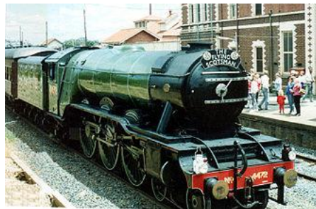
Flying Scotsman at Seymour railway station, Victoria in 1989, equipped with electric lighting and air brakes for operation on Australian railways.
