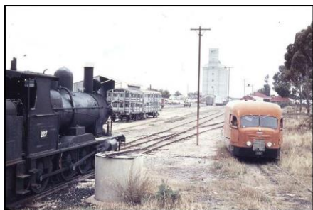
Taken in the late 1960s, a SAR Rx steam locomotive #227 with a Commer QX (R7) railcar #131 in the Karoonda rail yards. The petrol engine, Commer railcar operated the Karoonda to Peebinga service. The grain silos in the background were built in the early 1960s employing an eight-day continuous concrete pour. Source: Internet
